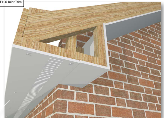
Fig. 16. Standard overcapping soffit installation.
