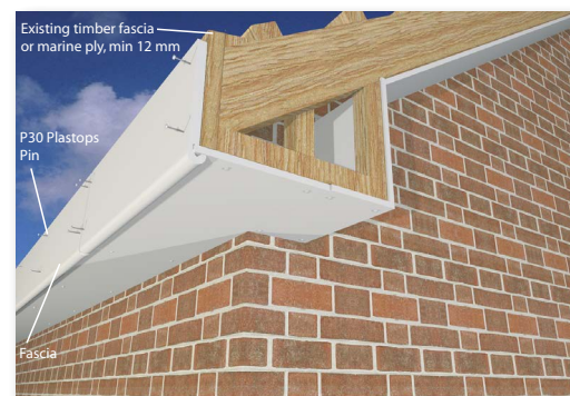
Fig. 17. Standard over-fascia installation.
