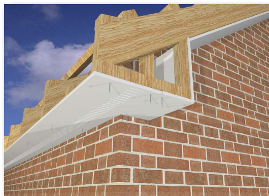
Fig 20a. Typical GPBV soffit installation.
