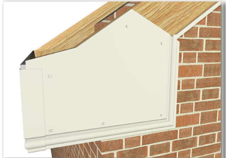
Fig. 27. Magnum Ogee Fascia box end configuration.
