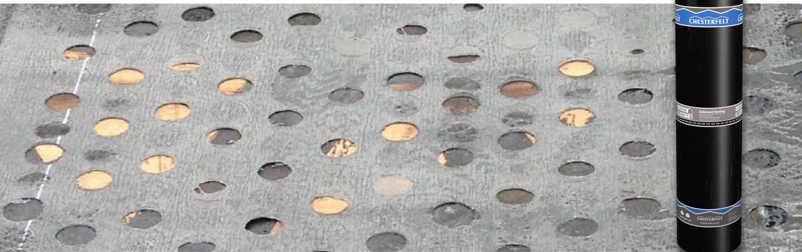
Debovent is a specifically manufactured venting base layer designed to be used as part of a multi-layer built up flat roofing system. It features a glass fibre core which is saturated and coated in bitumen and the upper surface is finished in a light sand.
