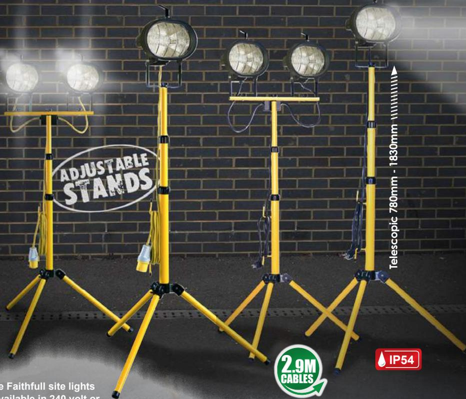
These Faithfull site lights are available in 240 volt or 110 volt and are supplied with 2.9 metres of cable and an adjustable tripod that adjusts between 780mm and 1830mm (31 and 72 inches). The fully adjustable head is fitted with a 400W halogen "C" class bulb that generates the same light as a conventional 500W halogen bulb, but using 20% less power.
