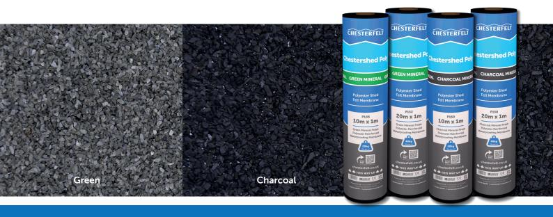
Chestershed Poly Mineral is a waterproof protection layer for use on portable type buildings with pitched roofs, such as sheds, stables, kennels and non-inhabited buildings. It features a polyester base which is saturated and coated in SBS modified bitumen and finished with light sand on the lower surface and mineral granules on the upper surface.
