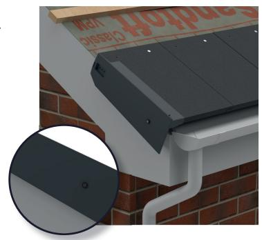
4) Screw through the central fixing hole into the centre of the tile batten using a 35 x 4mm stainless steel screw (supplied in the verge unit).
