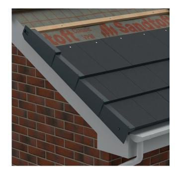
**Note:** When placing the unit ensure the flap is connected to the unit below as shown.
