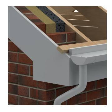
2) Lay the underlay in the usual way, allowing a 25mm overhang at the verge. Set out the tile battens at the appropriate gauge for the tile.
