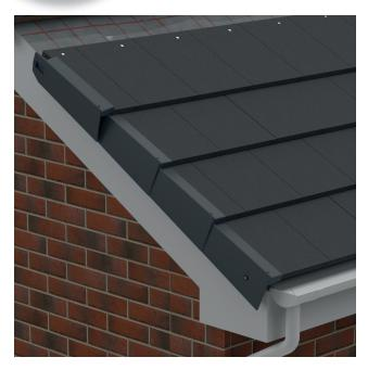
**5b)** Alternatively the unit can be slid into place prior to the next course of tiles.
