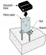
**Step 4:** Fix down the flitch plate to concrete foundation and lower the standoff over the flitch plate.
