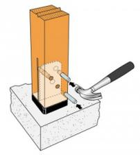
**Step 6:** Drive the dowels into the post. They should be roughly centred within the post.
