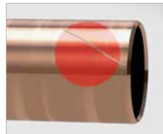
4. Check for scratches and scores
