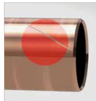
4. Check for scratches and scores
