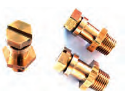
Test Nipples Brass screw connects gas meter to a gas test gauge. Hexagon screw shuts off supply to the gauge (1/8in.BSP).
