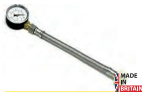
Mains Water Pressure Gauge 11 bar maximum. 3/4in BSP thread for fitting to taps. Tri-Scale kPa psi bar.
