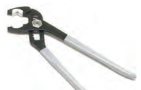
Soft Touch Pliers Soft jaws for use on as gold plated taps, stainless steel fittings etc to avoid damage. Five steps, easily replaced jaws fixed by recessed bolts (250x46mm Jaw).
