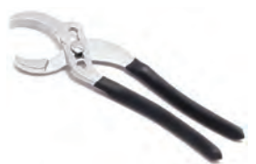
Wide Jaw Pliers Drop forged 5 position adjustment with toothed jaws for loosening and tightening round fittings on plastic waste pipes etc (250mm).
