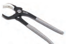
Wonder Pliers Drop forged with vinyl grips. 8 position adjustment. Spring action. With interchangeable round and square soft touch jaws for gripping delicate objects (270mm).
