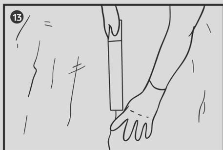
Join the individual sections of the vapor barrier film using overlapping silver adhesive tape.
