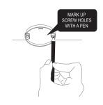
Use the mounting base ring to mark the screw holes on the ceiling or the wall.
