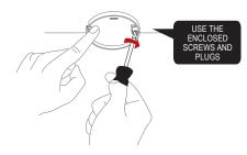
Once the mounting base is installed, attach the alarm by twisting clockwise until it clicks. If
