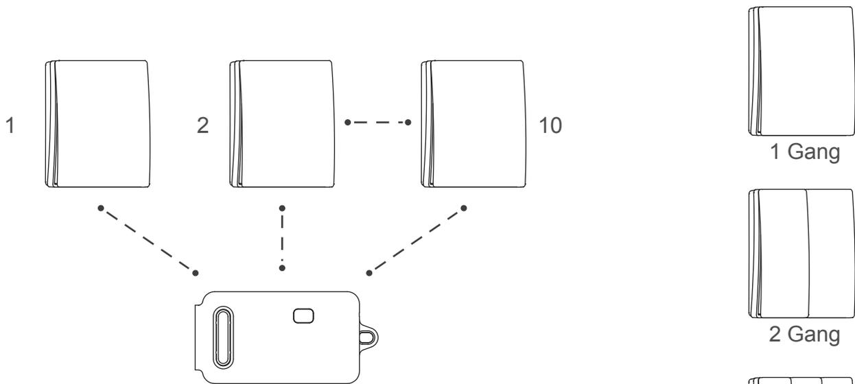
**Max. 10 Kinetic Switches to pair ONE On / Off Receiver.**
