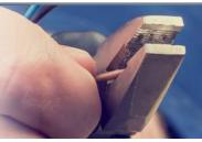
**Flectricians Pliers** Gripping and bending wire; crimping ferrules and cutting soft, medium
