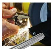
The 0.25 carat diamond tip is best suited for use on bench grinding wheels of up to 150mm diameter.
