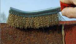
Popular with both industrial and DIY users, wire scratch brushes are used for removing rust, corrosion, paint and primer and for generally producing clean surfaces.
