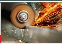
**N.B.** These metal CUTTING discs must never be used for grinding and must always be presented to the work piece at an angle of 90°.
