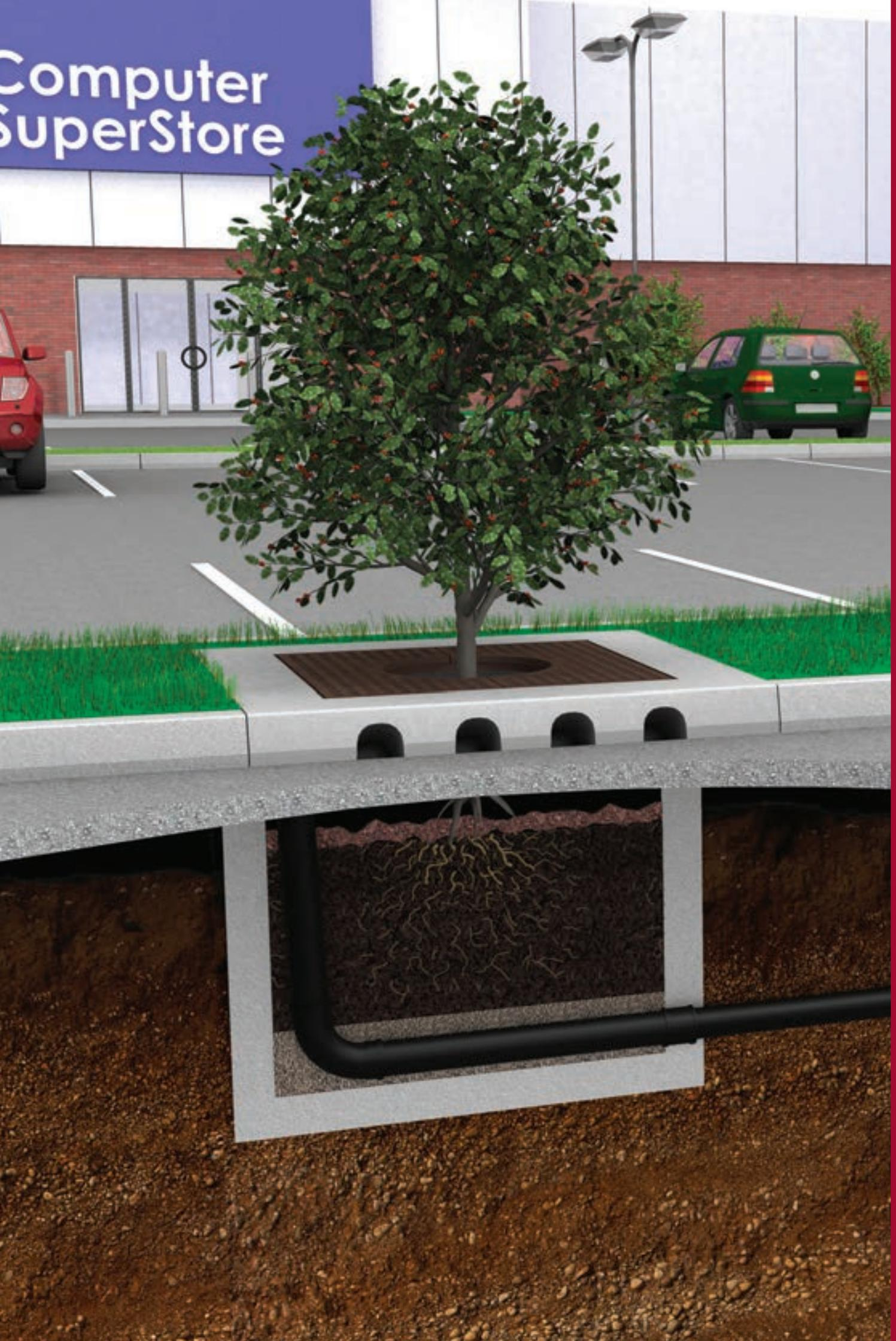
Biofilter™ Biofiltration System
