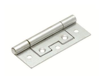
Flush hinge for lightweight applications such as cupboards. Has the advantage over a butt hinge as it fixes directly onto the surface without the need to cut a recess. Also the design allows one leaf to fit inside the other thus taking up less space. available in different sizes and finishes.
