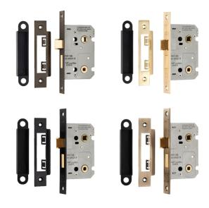
Contract Bathroom Lock with a wide range of options offering an excellent degree of choice. Square or Radius Forends, 64mm or 76mm sizes and 5 finishes. The Latch bolt has the Easi-T reverse function to save undoing the case so it can be reversed in seconds. Certified to BS EN 12209.
