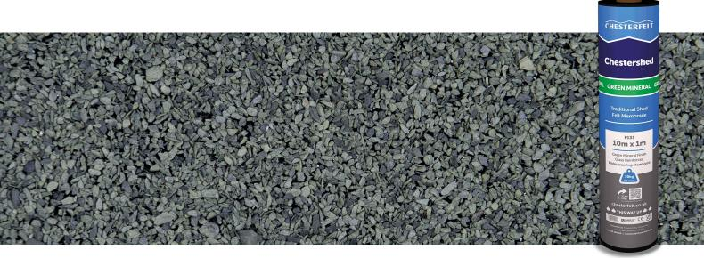
Chestershed Mineral is a waterproof protection layer for use on portable type buildings with pitched roofs, such as sheds, stables, kennels and non-inhabited buildings. It features a glass fibre base which is saturated in bitumen and finished with light sand on the lower surface and green mineral granules on the upper surface.
