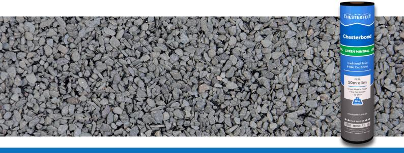
Chesterbond Green Mineral is a traditional pour and roll membrane which is used as the final waterproofing layer in conjunction with an underlay membrane such as Chesterbond Underlay. It features a rag fibre base which is saturated and coated in oxidised bitumen and is finished with light sand on the lower surface and mineral granules on the upper surface.
